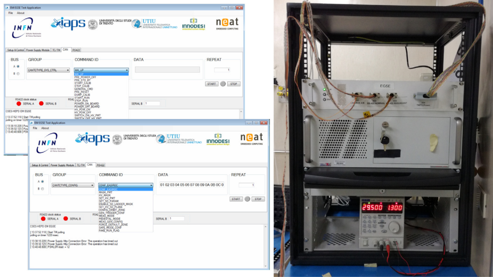
Fig. 6. EGSE: Electrical Ground Support Equipment, emulating the satellite, to manage HEPD configuration and acquisition (right). Screenshots of System Control and Configuration Telecommands are shown (left).
