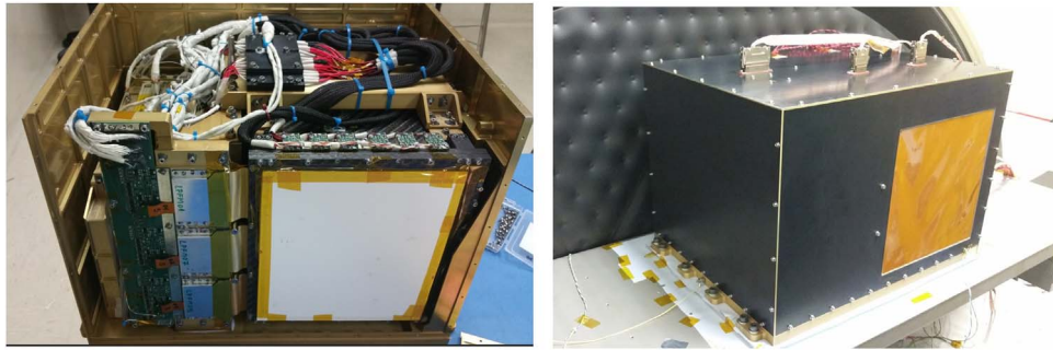
Fig. 6. Picture of the HEPD flight model (FM): assembly (left) and at the thermal-vacuum acceptance test (right).
