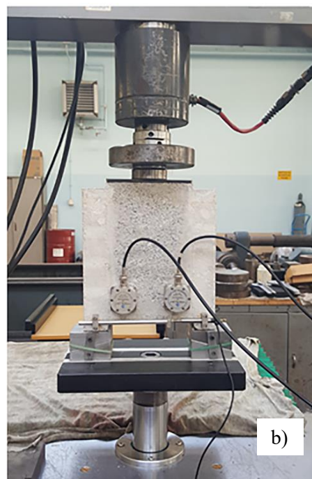
Figure 2. Geometry of composite specimen (a) and test setup (b).
