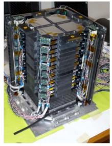
Figure 18. Picture of the assembled scintillator tower.
