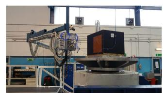
**Figure 7.** The HEPD-FM on the shaker system at the SERMS facility in Terni (Italy) in 2016 October.
