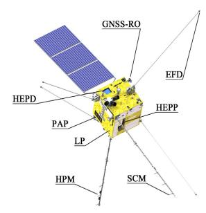
**Figure 2.** Position of the instruments on board *CSES*. The satellite is in orbit configuration, as shown by the deployed solar panel and booms.
