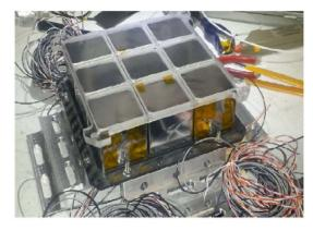
Figure 19. Left: emission spectrum of the EJ-200 plastic scintillator. Right: picture of the LYSO matrix plane.
