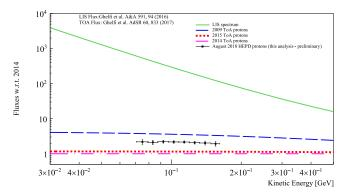
**Figure 16.** HEPD galactic proton flux (black squares) compared to TOA theoretical fluxes for 2009 (blue dashed line), 2014 (magenta dashed–dotted line), 2015 (red dotted line), and LIS spectrum (green solid line).
