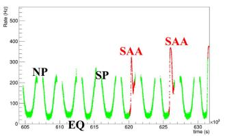
**Figure 11.** Top panel: HEPD average event-rate map during the period from 2018 May 14 to June 11. The red spot around Brazil represents the SAA, in which the rate counter saturates at about 350 Hz. Bottom panel: HEPD trigger rate as a function of onboard time for a few orbits. Different regions are marked.
