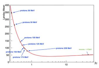
**Figure 9.** Calibration curve of one tracker ladder of HEPD. On the *Y*-axis, the mean of the Landau distribution of the energy deposited by the beam test particles at a given energy is reported. Also, one point obtained by cosmic-ray muons is shown. The red line is the theoretical Bethe curve.
