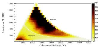
**Figure 13.** In-flight proton–electron identification by HEPD: energy released in the first plane of the calorimeter (P1) as a function of that released in the full calorimeter (P1 + ... + P16).
