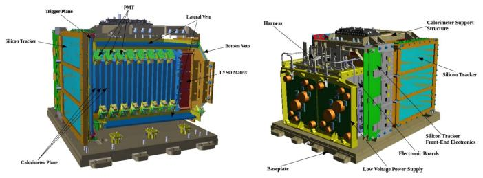
Figure 6. Schematic views of the HEPD electronics box and detecting units.
