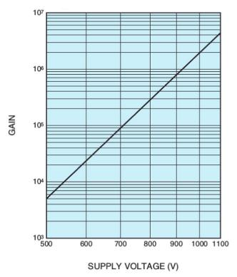
Figure 20. (Left) PMT quantum efficiency and (right) gain.
