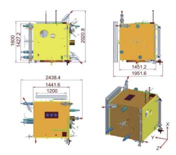
Figure 1. Layout of the CSES with stowed solar panel and booms.
