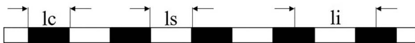
Figure 2. Recording electrode. Representation of a portion of a Dixi electrode adopted in the majority of the MNI channels investigated, with the typical dimensions: length of contact (lc) \sim 2 mm, distance between consecutive contacts (ls) \sim 1.5 mm, resulting distance between the centres of two contacts (li) \sim 3.5 mm. The total exploration length depends on the number of contacts of an electrode varying from 5 to 18 in the studied recordings.
