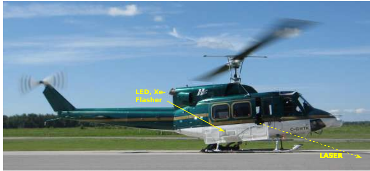
Figure 3. The light sources were mounted on a Bell 212 helicopter.
