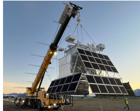
Figure 1: Entire payload hanging off the launch crane, attached to the balloon minutes before takeoff.
